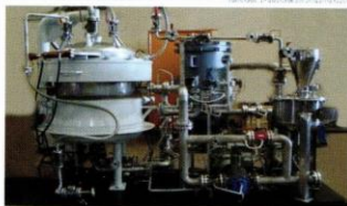
Skid mounted unit with piping and valves
