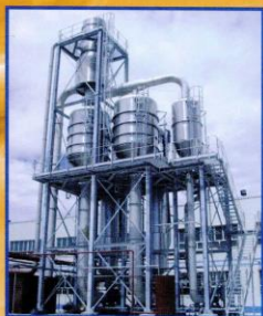
Triple-effect forced circulation evaporator For fruit puree - China
