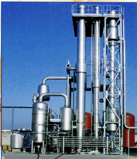
Multi-effect falling film evaporator For fruit juice - Italy
