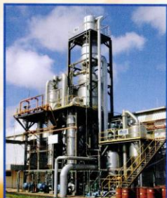
Triple-effect forced circulation evaporator with HB system For tomato paste - Brasil
